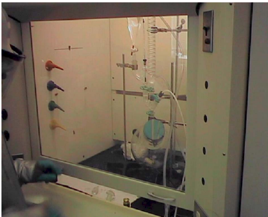
Figure 3. Set-up for converting sodium superoxide to sodium alkoxide.
